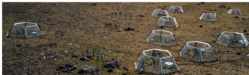
Figure 1. Visualization of an OTC chamber used in the experiments in order to simulate the day time warming and a photograph of a measurement spot (King George Island, South Shetlands), with OTC installed.
