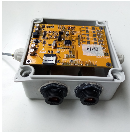
Figure 7. The ARM-Node inside IP67 enclosure. The rugged RJ45 connectors and cable glands are show.
